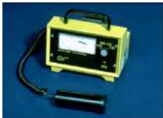
FIG. 62. Compensated and end window dose rate meters
