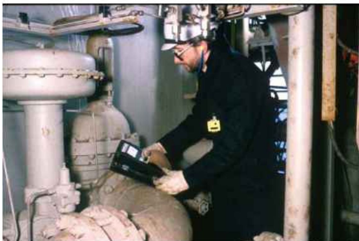
FIG. 48. Monitoring the outside of plant and equipment using a dose rate meter (Courtesy: HPA-RPD, UK)
