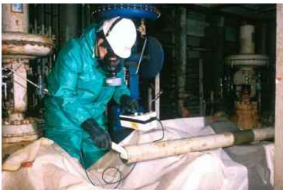
FIG. 72. Checking tubulars for NORM contamination (Courtesy: HPA-RPD, UK)
