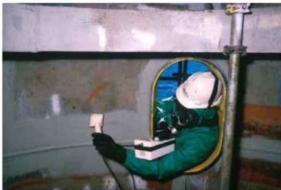
FIG. 71. NORM contamination within a vessel being measured using a surface contamination measuring instrument (Courtesy: HPA-RPD, UK)
