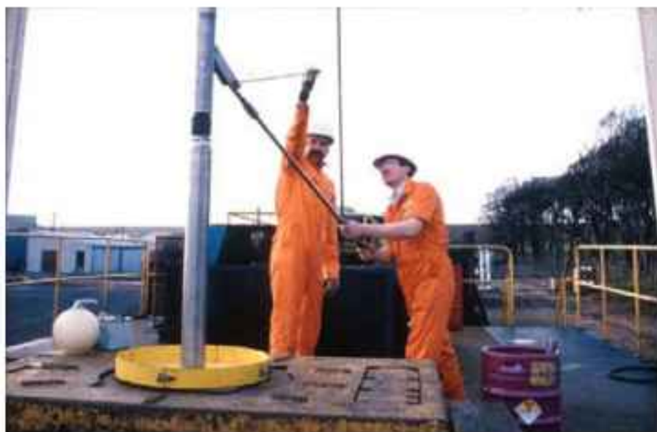
FIG. 21. Wireline engineers transferring radioactive sources to logging tools on the drill deck (Courtesy: HPA-RPD, UK)
