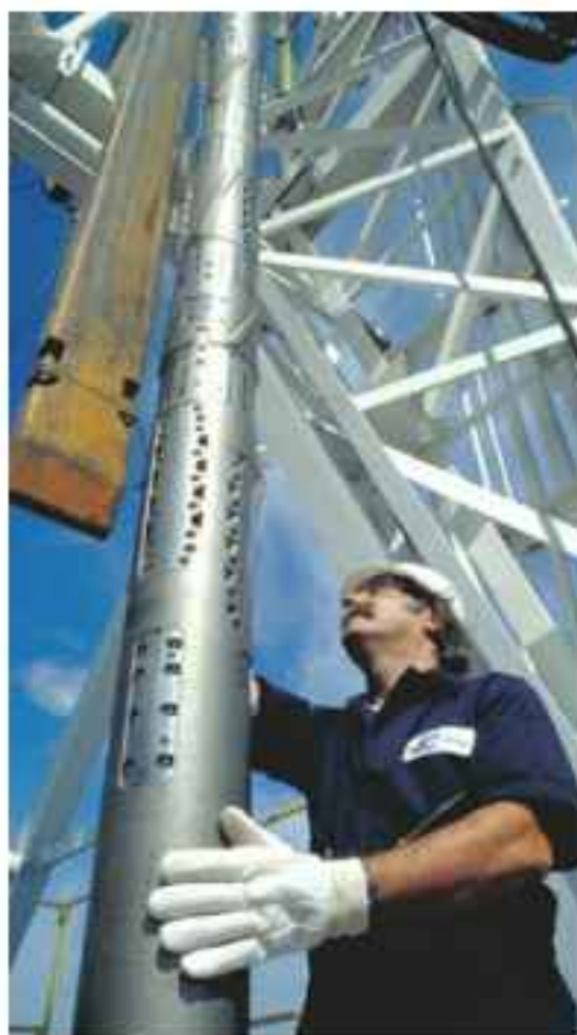
FIG.18. Well logging tool string suspended by a derrick above an oil well (Courtesy: Baker Hughes INTEQ)
