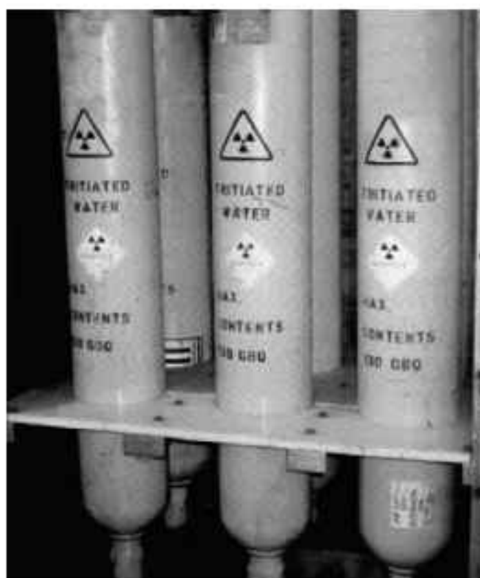
FIG. 26. Tritiated water for injection as a radioactive tracer (Courtesy: Scotoil Group plc)
