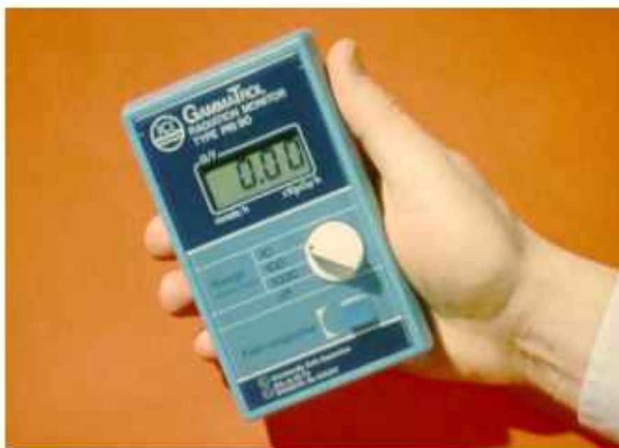
FIG. 64. Intrinsically safe dose rate meter
