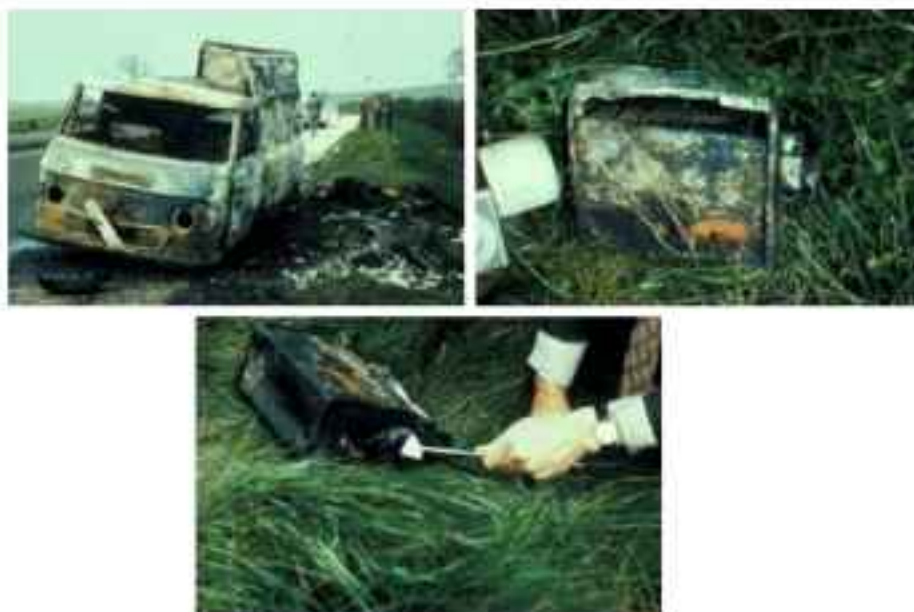
FIG. 78. Damaged radiography source after vehicle fire. The shielding was still intact and smear tests showed no apparent leakage of radioactivity.
