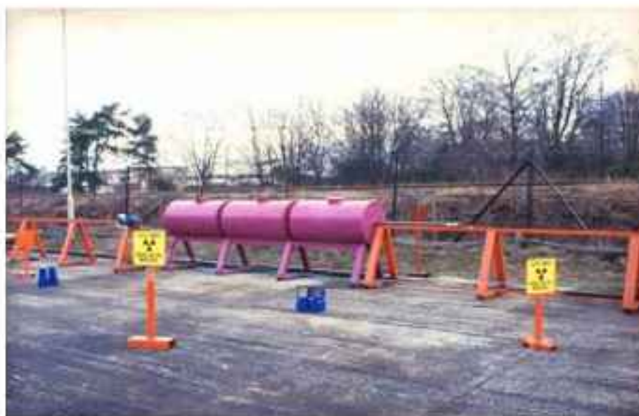
FIG. 23. Controlled area in which low dose rate radiation test sources are used during tests in the workshop (Courtesy: HPA-RPD, UK)
