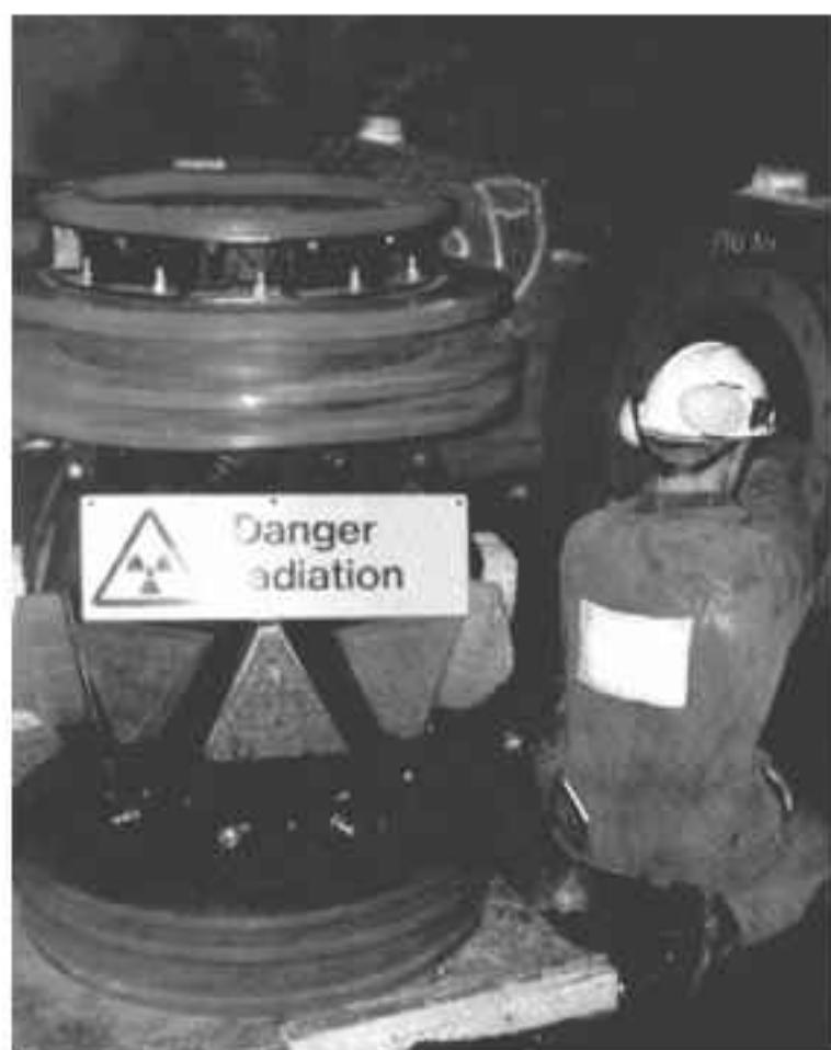
FIG. 17. Radioactive sealed sources incorporated in a pipeline pig (Courtesy: Scotoil Group plc)
