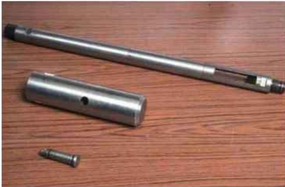
FIG 24. Gauge for measuring the density of well fluids (Courtesy: HPA-RPD, UK)
