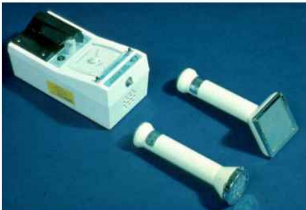
FIG. 70. Portable contamination rate meter with beta probe and alpha-beta dual probe
