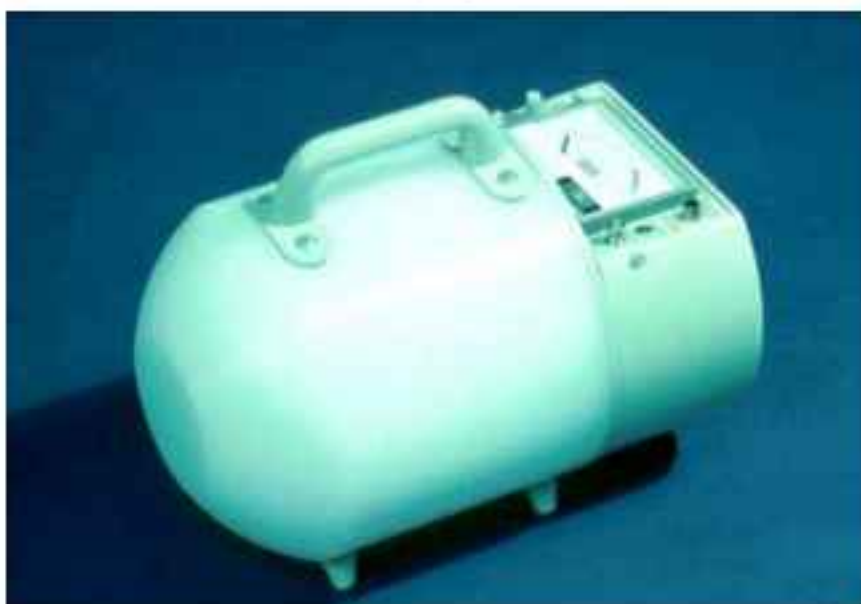
FIG. 65. Neutron dose rate meter (17 MeV energy response)
