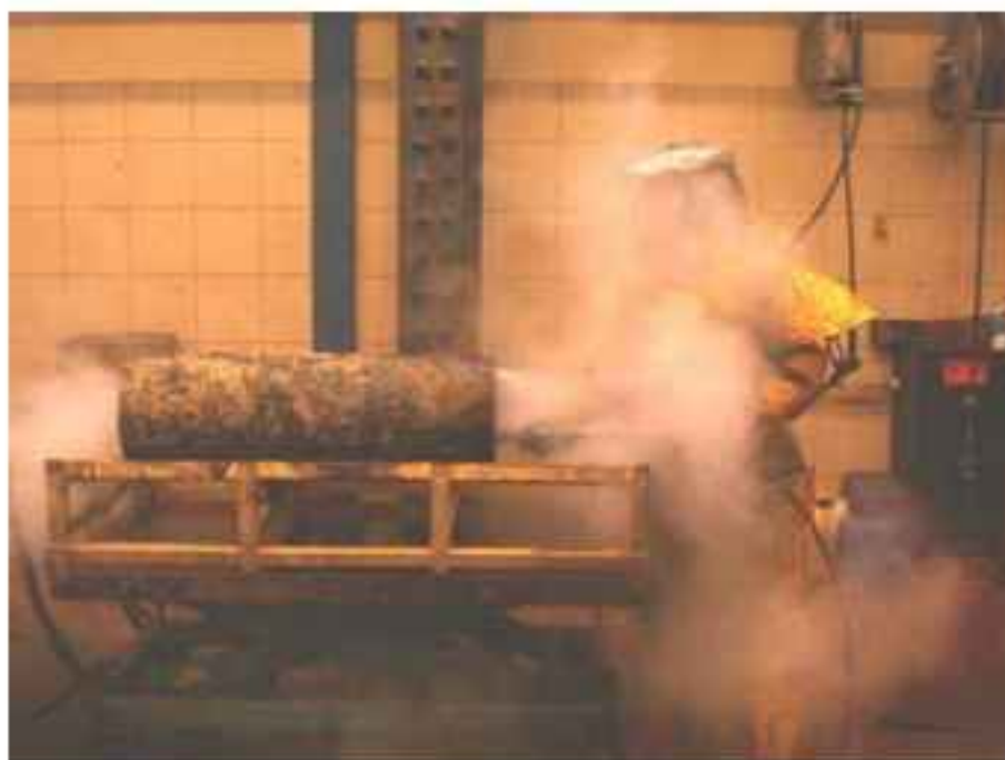
FIG. 55. Worker using a HPWJ lance (Courtesy: Atomic Energy Commission of Syria)
