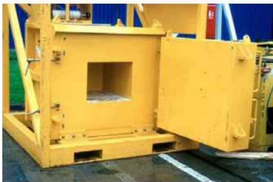
FIG. 20. Transport container used as a temporary store for well logging sources (Courtesy: HPA-RPD, UK)
