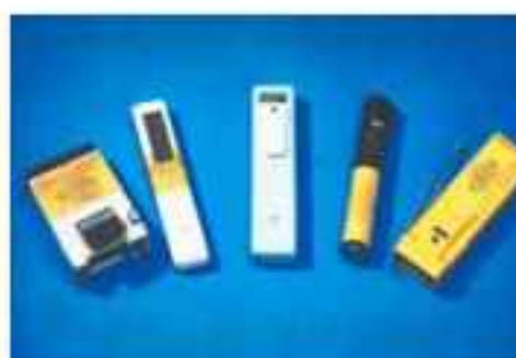
FIG.68. Direct reading dosimeters: quartz fibre electrometer (left) and electronic dosimeters (right)
