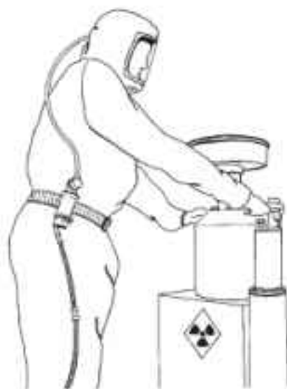
FIG. 40. A full suit supplied by compressed air line
