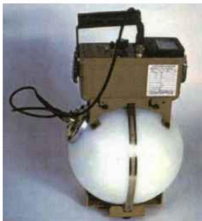
FIG. 66. Neutron survey meter (10 MeV energy response)
