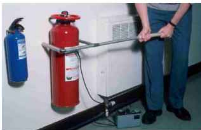
FIG. 16. Mobile gauge for detecting the level of liquids in closed fire extinguisher cylinders (Courtesy: HPA-RPD, UK)
