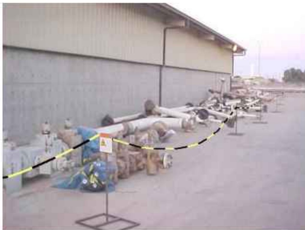
FIG. 51. Barrier designating a controlled area to restrict access to NORM-contaminated equipment stored outside a decontamination facility (Courtesy: HPA-RPD, UK)
