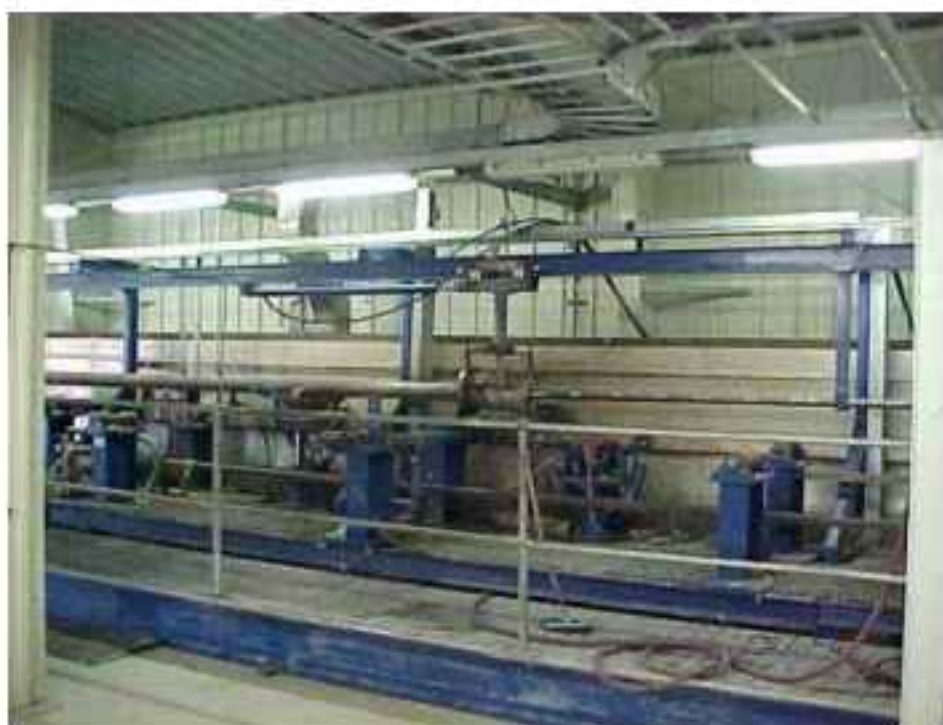
FIG. 56. Facility for tubular decontamination by HPWJ (Courtesy: Atomic Energy Commission of Syria)
