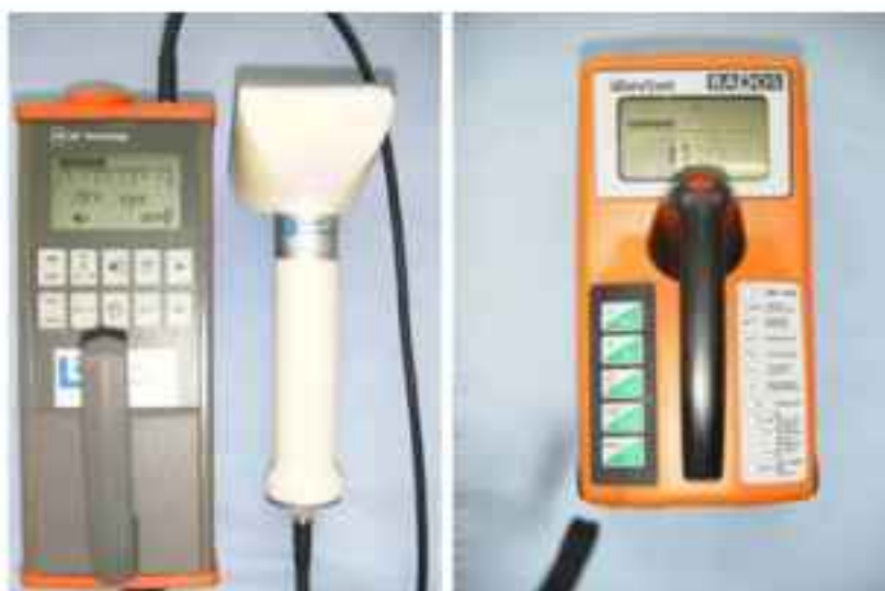
FIG. 69. Two types of surface contamination monitor
