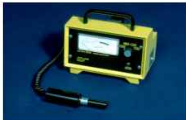
FIG. 62. Compensated and end window dose rate meters
