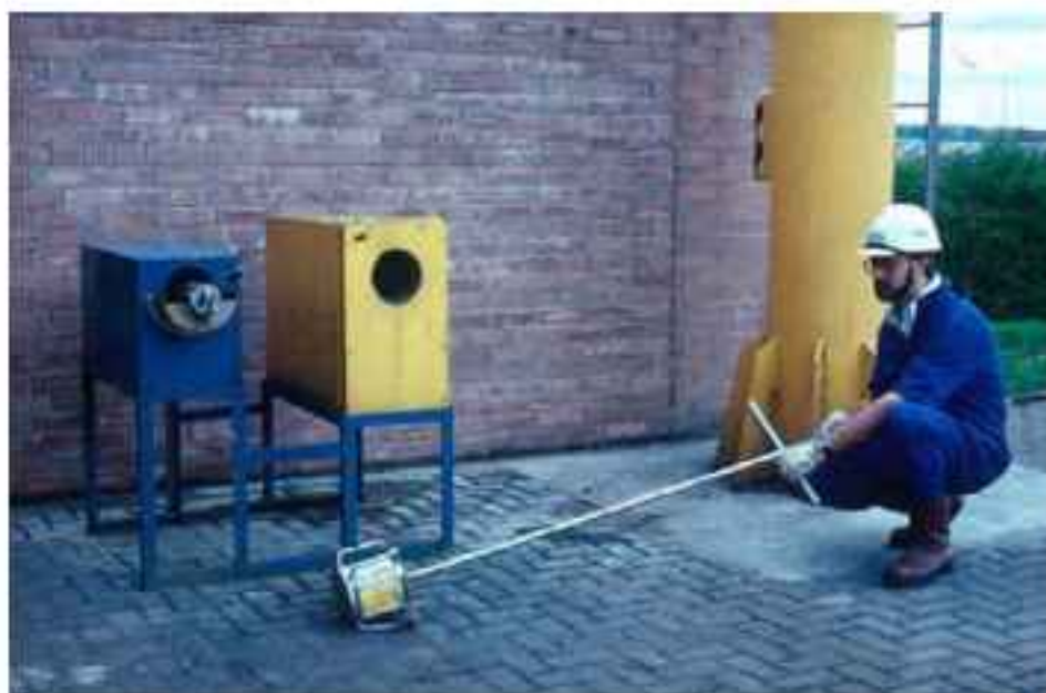
FIG. 22. Wireline engineer using a handling tool to transfer a radioactive source during a calibration procedure (Courtesy: HPA-RPD, UK)
