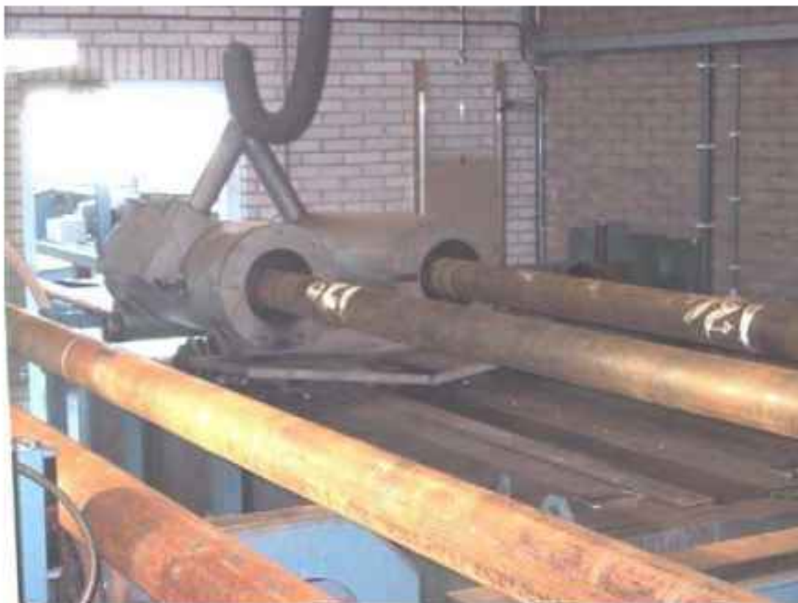
FIG. 53. Dry drilling of tubulars with a closed extractor system to remove contaminated dust (Courtesy: Atomic Energy Commission of Syria)
